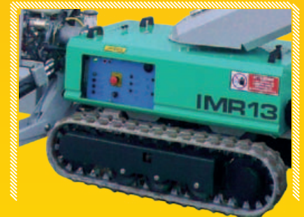
Ground control panel easy to access and protected inside frame guards
