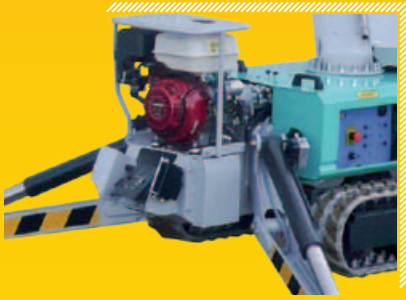
Endothermic power pack duly guarded for improved safety
