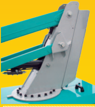
Rotating turret hosting hydraulic components of the platform's aerial section
