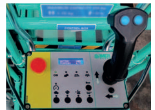
Control panel on the platform with capacitive buttons: simplicity and safety of use
