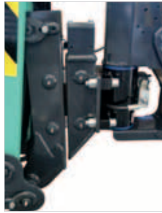
Compact jib group with load cell and basket rotation system.
