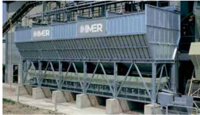
Aggregates storage unit ORU ROME CZ
