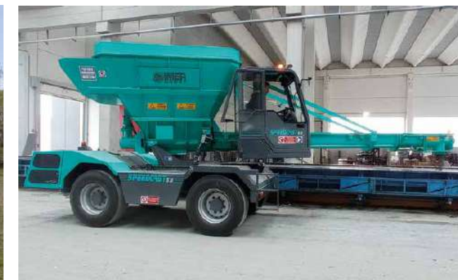
SPEEDCAST SCC concrete casting phase in horizontal formworks
