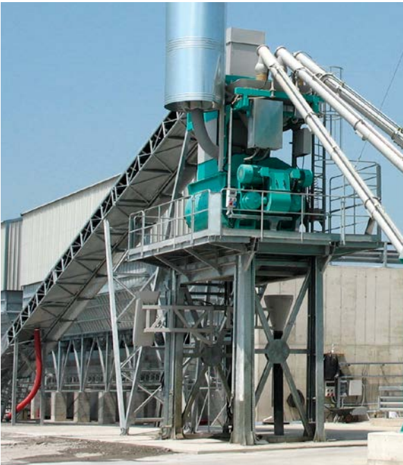
ORU LK 100-120-125-130 mixing unit with loading belt and aggregate waiting hopper.
