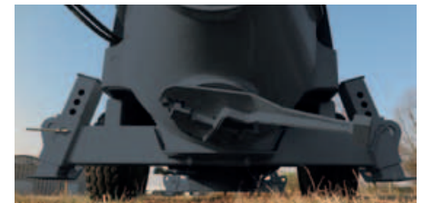
Hopper unloading door.
