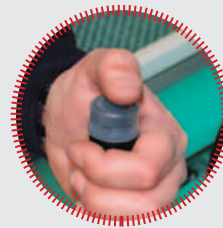
Cooling air flow diverter of the mixer motor, to avoid the spread of dust in the work environment during bag loading.
