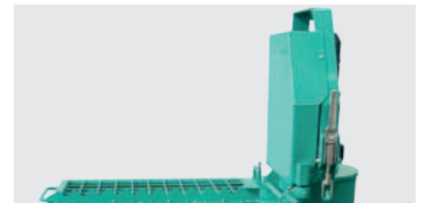
Cooling air flow diverter of the mixer motor, to avoid the spread of dust in the work environment during bag loading.
