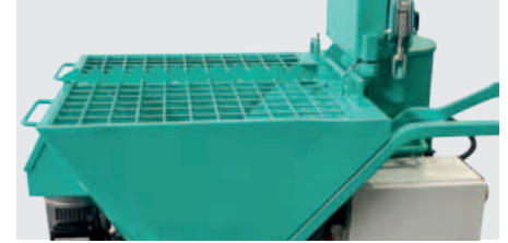
Grate with bag breaker.
